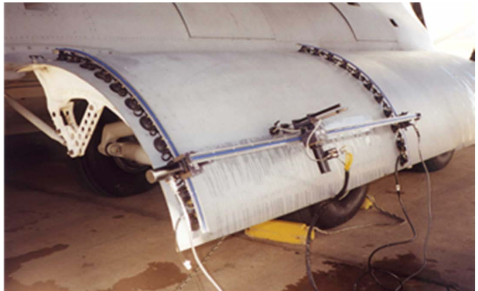
Catamaran scanner mounted on a C-17 landing gear cover.
